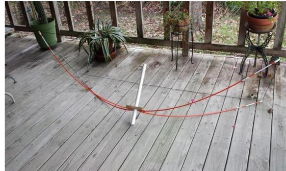
Disconnect the diagonal strings when you're done if you haven't already thrown them as far as you can. The antenna can now be assembled or disassembled very quickly since there are no bolts or screws holding it together. There is also no need to remove the PEX end caps from the wire elements at this point. Pop the end caps off the spreaders and pieces will begin to fall on the ground. Gather up the pieces, stuff them in a bag, and you're portable.
